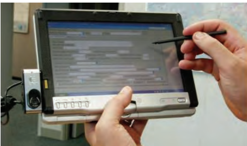
Figure 21. Screeners in the field used computer tablets for data entry. Screeners used a digital camera (attached to tablet at left) to take photographs of buildings and irregularities.
