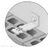
Examples of veneer anchors. There are many proprietary types available.
