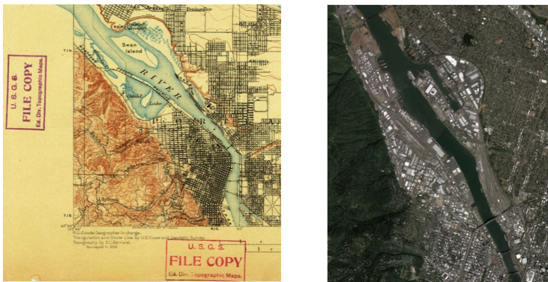
Figure 2-1. Reclaimed land through engineered fill in the CEI hub area (a) Portland-area map showing historic lakes that underlie the CEI hub (USGS 1901), (b) satellite view of the Portland-area (image dated 13-August-2020 from Google Earth).
